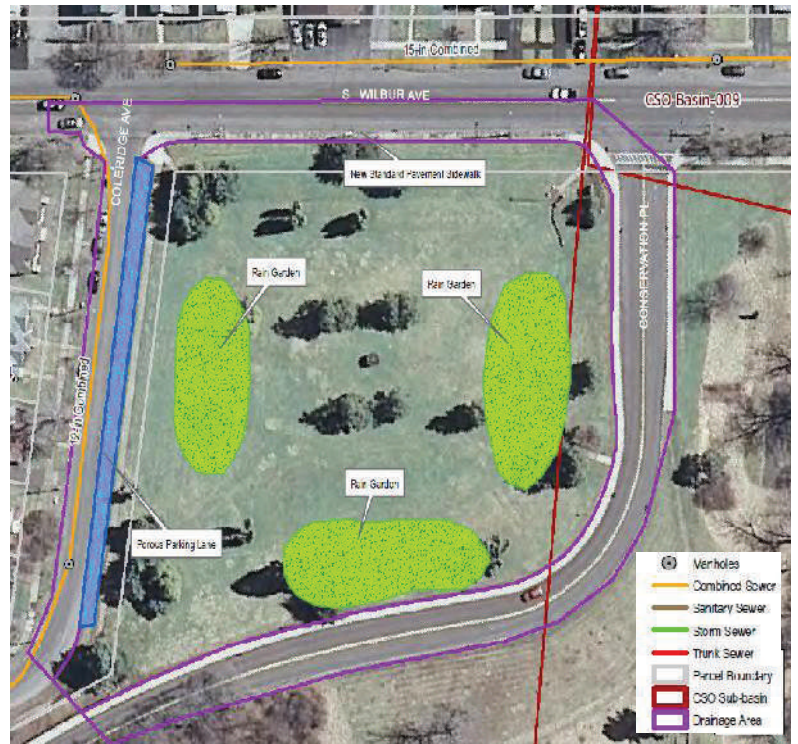
Conceptual Rendering of Wilbur Ave. Zoo Entrance Green Infrastructure (Courtesy: CH2M Hill)
