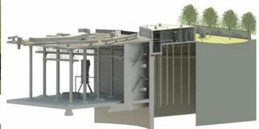
Rendering – Cross Section of Underground Storage Facility
