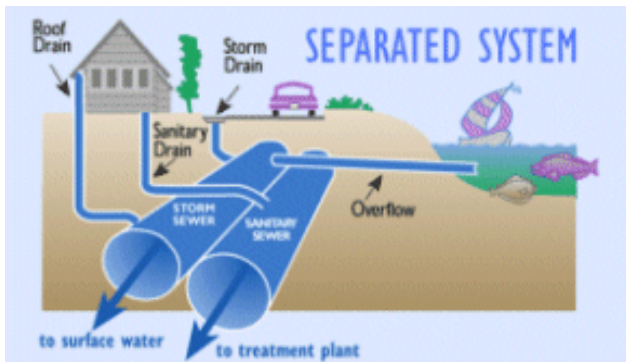
Schematic of Separated Sewer (EPA)
